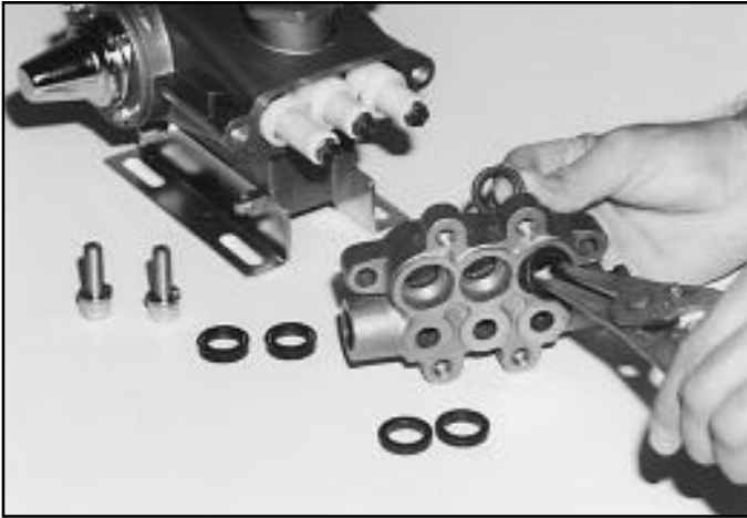
Removal of Hi and Lo-Pressure Seals
