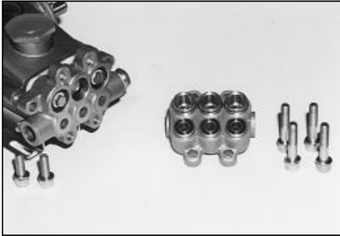
Removal of Discharge Manifold and socket head screws
